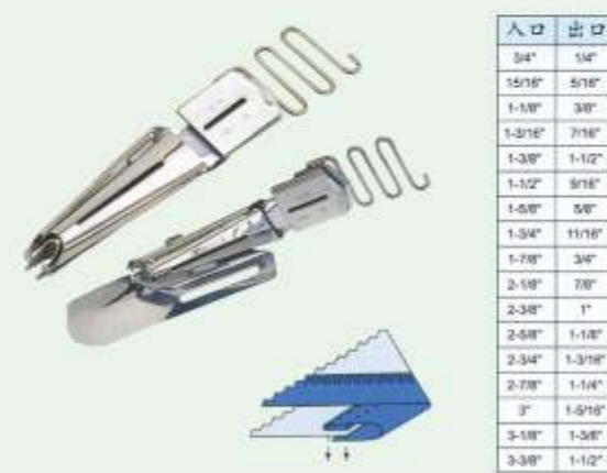
JZ-15510 K710NA(A)(F402) 绷缝车直角包边筒 (插口单折可调) Right Angle Binder K712NA(A) 绷缝车直角包边筒 (平口单折可调) Right Angle Binder
